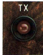
TX LIGHT indicates transmitter is keyed.
